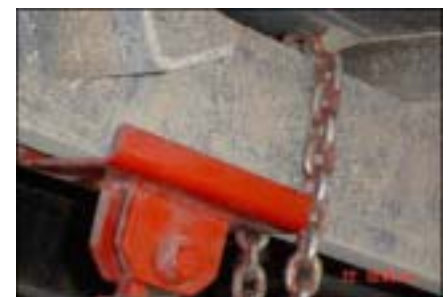
Figure 3 shows the top channel of the truck bed brace bracket. These braces also have a handle that allows an employee to place the brace under the dump box without creating an additional hazard.
